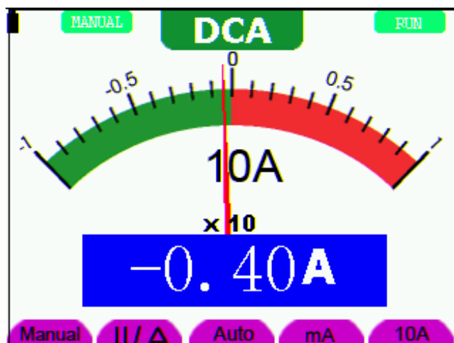
Figure 28: DC Current Measurement for 10A
