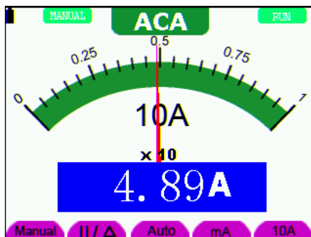
Figure 30: AC Current Measurement for 10A
