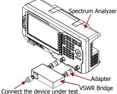
Connect the device under test
